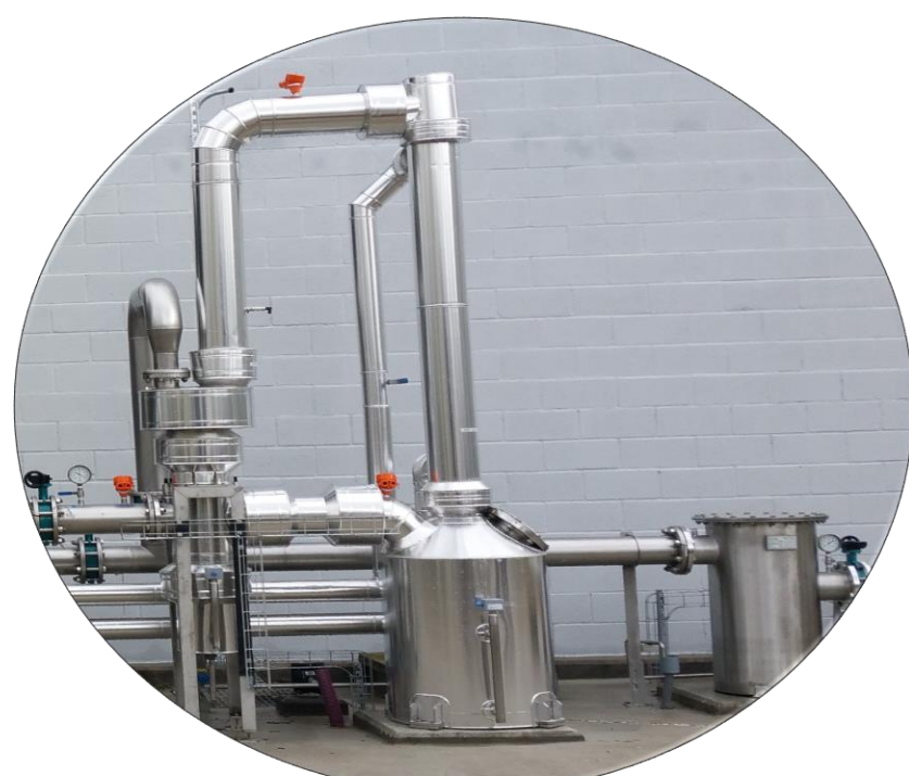
Figures 4. Dryer. Vertical position with energy recovery
